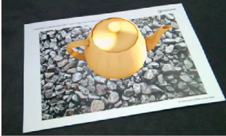
Figure 4.1: Example of Hologram projected using image target; via https://library.vuforia.com/articles/Training/Image-Target-Guide
