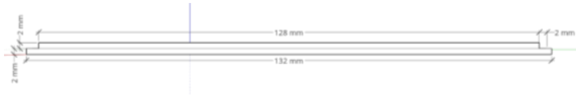
Figure 27. Front View of device back cover
